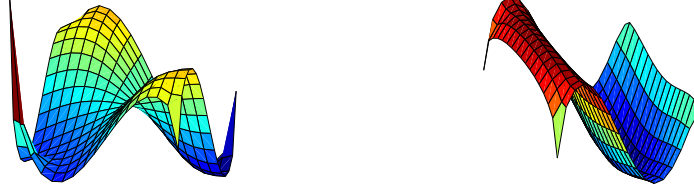
FIG. 4.1. Extension of the coarse level primal finite element basis functions to the interior of a subdomain: extension of a corner basis function (left); extension of an edge average basis function (right).
