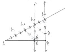
Draw any ray starting at A lopy a regnent of any length 4 times along the ray. Draw a line parallel to \$\overline{A}\_4 B\$ through \$\overline{A}\_5 A\_2\$, This line intersects \$\overline{A}\_8\$ at \$X\$ and \$\overline{A}\_X = \frac{3}{4} AB\$ by nimilar triangles.
