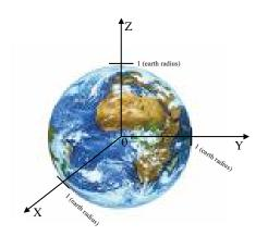
The GPS receiver is on a boat and receives simultaneously from 4 satellites their position in relation to the xyz-coordinate system (units radius of Earth) and the time the signal was sent in milliseconds. The data is given in the table below. The numbers are fabricated so that they are easy to manage, but they not completely unrealistic.
