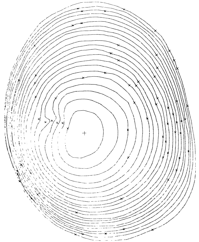
Figure 4 Contour map with concave areas indicated by x .
